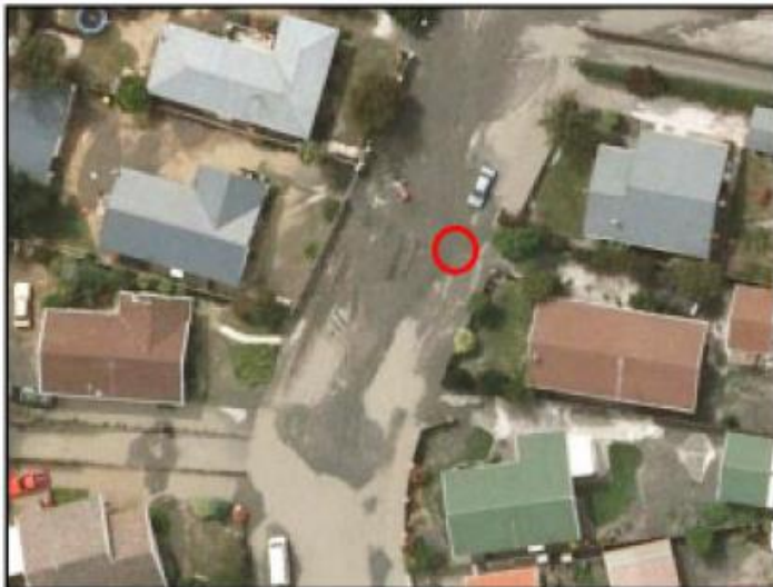
(c) Severe Liquefaction
